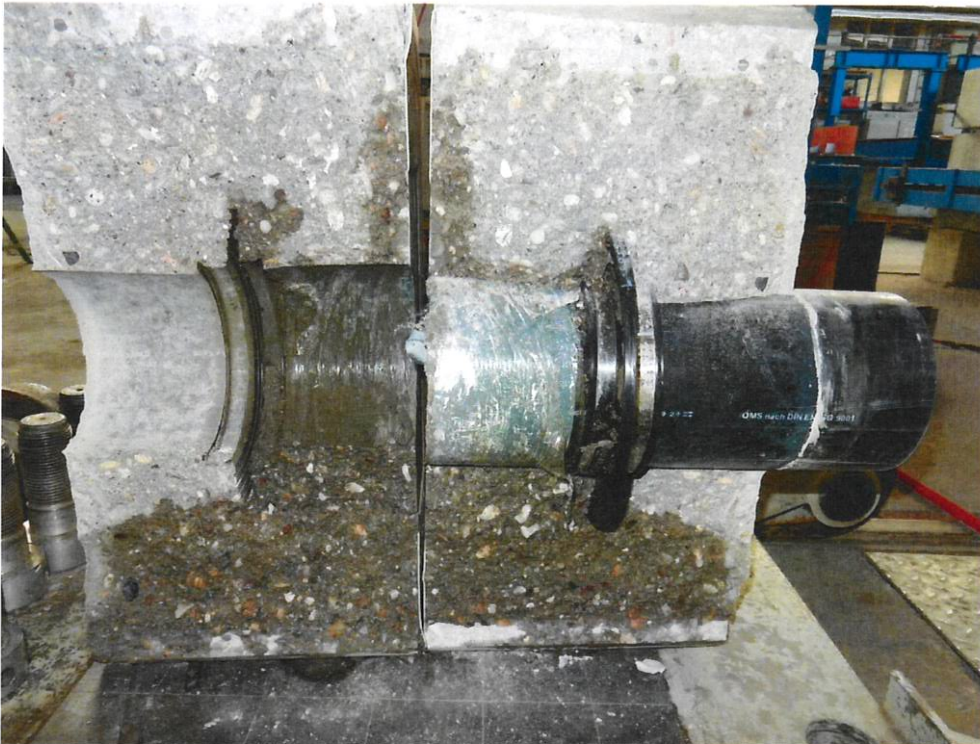
Figure 5 Split test specimen; inside: Water side; outside: dry side sealed by the sealing collar; extended spread at the bottom due to run-off residual water during splitting
